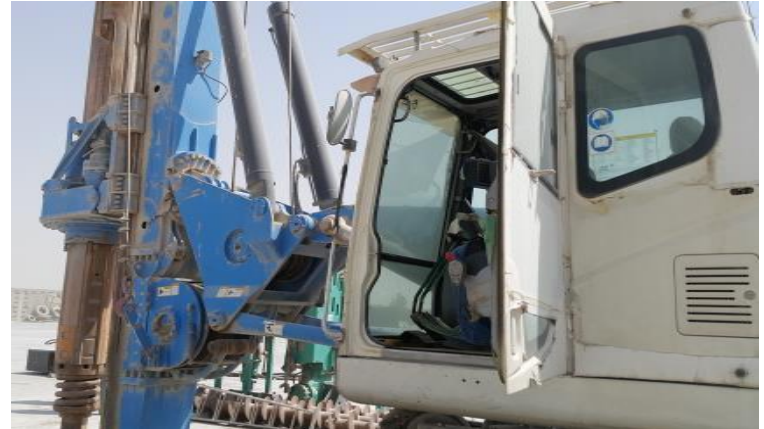
HYDRAULIC PILING RIG (SANY SR200C)
